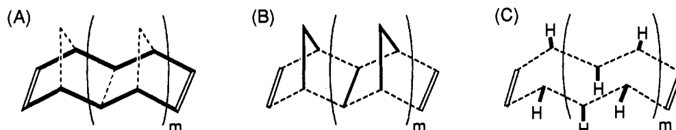
Figure 1. The three major components that affect the electronic coupling in 3(n) are the following: (A) the two alkyl relays connecting the two chromophores (highlighted bonds); (B) the cross-links connecting the two alkyl relays (highlighted bonds); (C) the C–H bonds adjoining the two alkyl relays (highlighted bonds).
